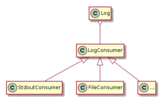
Log is the entry point of the Logging system. It exposes three macro definitions to ease its usage:
